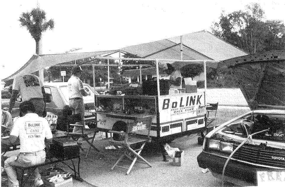
BoLink's New Race Trailer has four separate pit spaces and each can be separately locked, There is a power hook-up and lights for each space run from a 280Ah battery.
