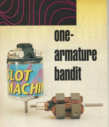
RINITY'S\* NEW Slot Machine was the first motor to be approved under the 1991 ROAR rules requiring that stock-class motors have locking devices on their commutators to restrict timing to a maximum of 24 degrees. The fixed commutator prevents racers from tampering with the motor's timing—a too-common practice at large-scale R/C racing events.
