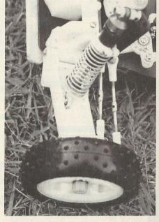
The universal drive shafts on an RC10 tend to bend but Traxxas have adopted the Schumacher method which is more reliable
