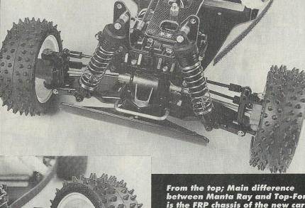
between Manta Ray and Top-Force is the FRP chassis of the new car. Standard shock absorbers are more than adequate - Hop-Up options are available though. Front and rear gearboxes are the same as the Manta Ray, Shock brackets are in FRP though - an improveement over the earlier car. Universal joints are employed in the front hubs. Do not apply grease here - it's a dust magnet!
