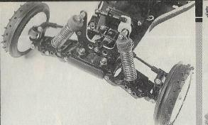
Ground clearance on the car is reasonable but damping and springs seem a little light. New steering hubs are part of the new handling package.
