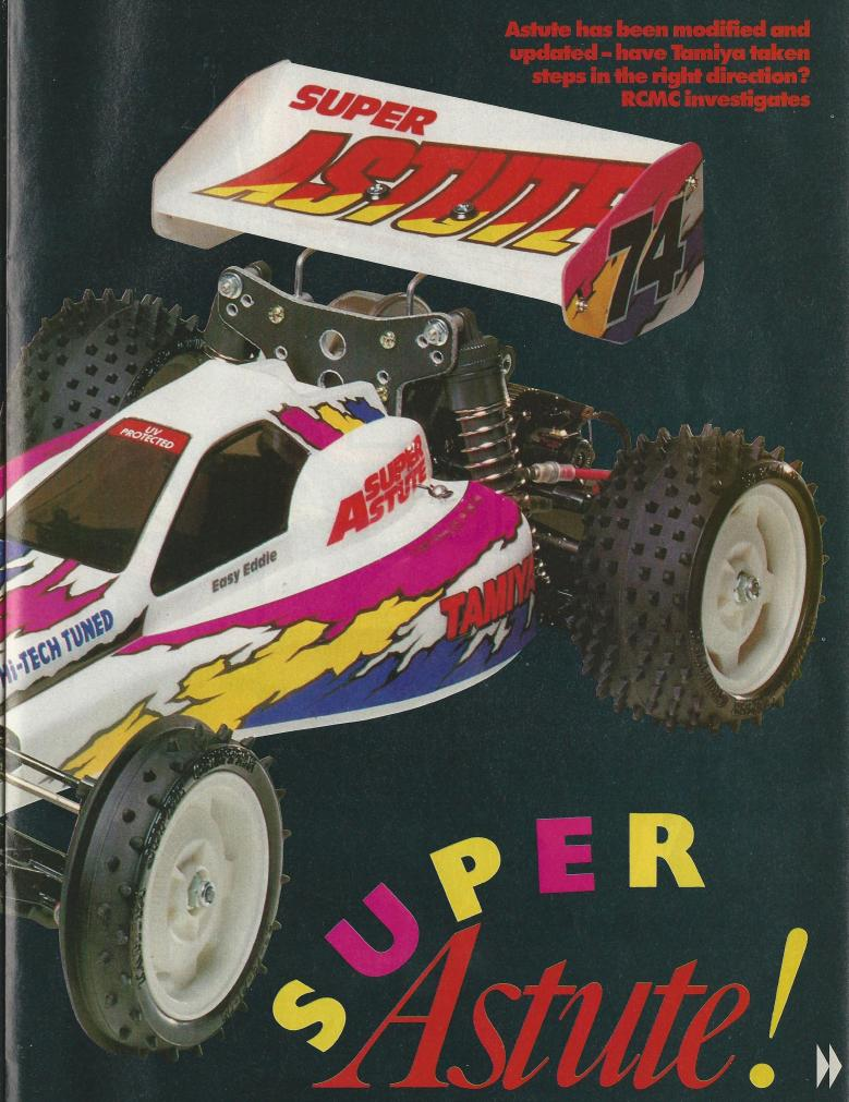
Below; Rear wing on Super Astute bolts together and is adjustable. Neat petite body gives Astute a racy look. New wheels and tyres are light and grippy.
