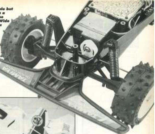
**Suspension is simple but effective - servo is a separate unit to the speed controller. Wide front bumper helps against damage.**
