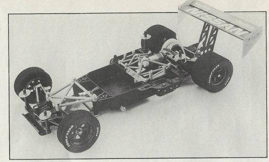
just a flat piece of G.R.P. Suspension movement is obviously limited and is controlled by small coil springs at the front and an oildamped flexible rear motor pod at the back.
