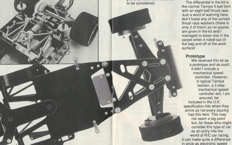
oil filled shock absorber. This arrangement is very similar to those used on other PRO-10 style cars as well as 1/12th circuit racers. It is a very simple setup whereby torsional movement of the T-piece is governed by an O-ring which can be compressed by tightening a screw through the T-piece and into the chassis. As a general guideline, more steering can be achieved by tightening up this screw and vice versa.
