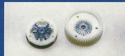
Differential gear assembly. Requires a bearing washer at each end - see text.
