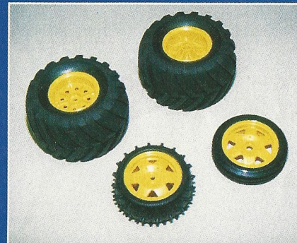
Mad Bull monster boots, compared with replacement Fighter Buggy tyres used for Cadet racing.
