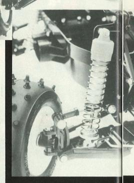
The King Cab has excellent suspension that actually works! The car handles well with lots of chuckability. The front anti-roll bar keeps the car level during cornering. Bathtub chassis probably has more room for R/C gear that anything we've seen before. Ball diff. and 540 motor add to the performance. to the performance.
