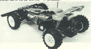
The old 'Hotshot' suffered from a large degree of 'bumpsteer', this it was felt was the answer to the understeer problem, but the 'Hotshot II' even with the same steering set-up seems not to suffer. The car has initial good turn-in followed by a slight power on understeer which certainly
