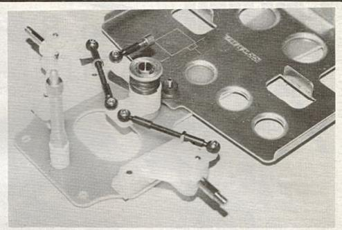
Above left: assembled differential with alternative fixed gear alongside. Above right: very nice substantial trackrods: and adjustable servo saver. High castor angle front-end follows fashion.
