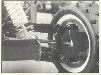
rod, eliminating those fiddly E rings that invariably end up in the Hoover or the dog! All the necessary oil is supplied and Loctite is a thing of the past as the self tapping screws used throughout are easy to drive home. Tyres are of the pin spike pattern but the choice of alternatives is endless. A mechanical speed controller is included so all you need is a budget two
