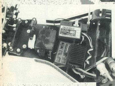
Above: Glassfibre shock mounts have various mounting positions. Radio installation is simple, but electrics must be kept low to avoid the bodyshell. Bottom: Front suspension detail.
