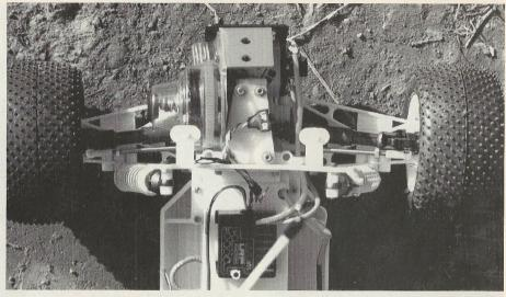
The rear end also utilises RC10T wishbones and Traxxas shocks, this time with Losi pink soft springs, hung from an RPM RC10T truck bulkhead. The rear uprights are from the Losi truck, as are indeed the slider driveshafts.
