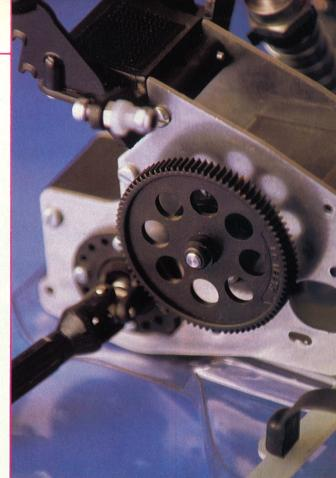
One way roller clutches are used on the front of the Procat.
