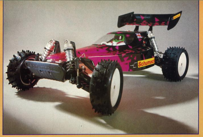
three days 4WD racing at the Worlds. The pivot pins for the rear suspension work out of their mounting during racing. The inner one works out of one hole, and the outer one works along the upright until it rubs against the wheel. The cure was to apply a large 'blob' of super glue to each end of each pin and the problem went away. The other problem was the use of TOPCAT wheels, which flexed so much on landing from the large jump on the Sydney track, (a jump taken
