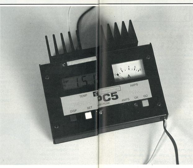
The setting of the thermal probe cut off is very easy. Two buttons are supplied, DISP (display) and SET. The LCD display reads the current probe temperature continuously which will be the surrounding air temperature unless inserted in a pack. Pressing DISP allows the user to operate the SET button to feed in the required cut off temperature. This must obviously be higher than the current air temperature or the unit will not even be able to switch on!
