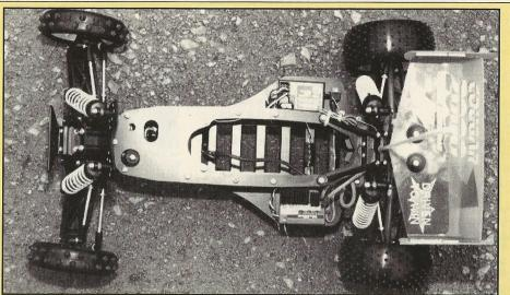
amount of toe in, but also the height of the axle line in relation to the suspension pivot point, yet another 'tweak' to play with! The wheel base can be adjusted at the rear, by spacer washers placed either in front of or behind the uprights, between them and the mounting points at the outer ends of the wishbones.
