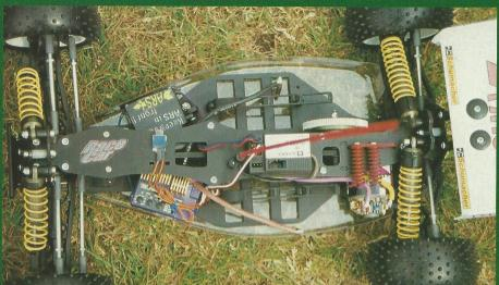
Schumacher have again kept their easy adjustable pistons, which offer a choice of one to four holes to alter the damping without changing the oil. Again, two types of O ring seals are supplied, red and white, but be warned, the low-drag white ones can leak slightly.
