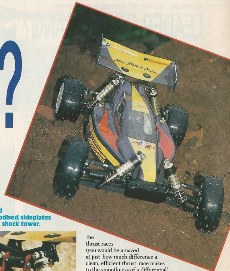
New rear end including anodised sideplates and graphite shock tower.
