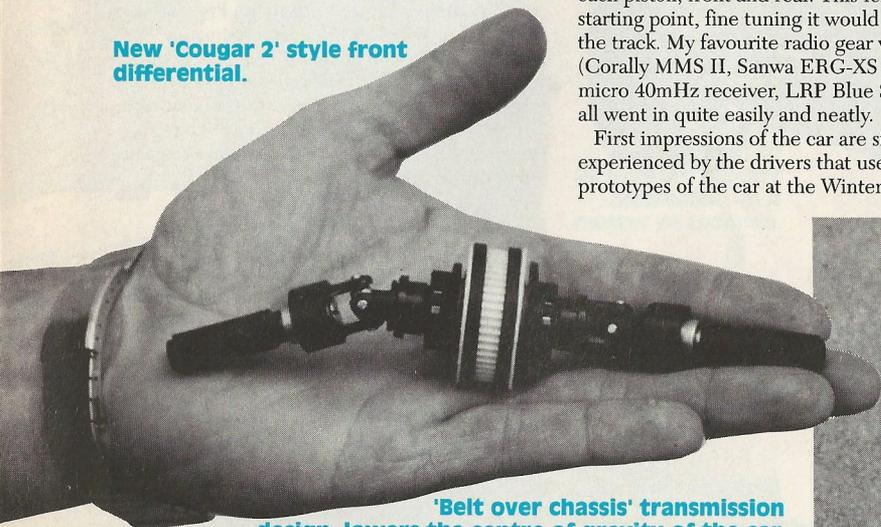
'Belt over chassis' transmission design, lowers the centre of gravity of the car.
