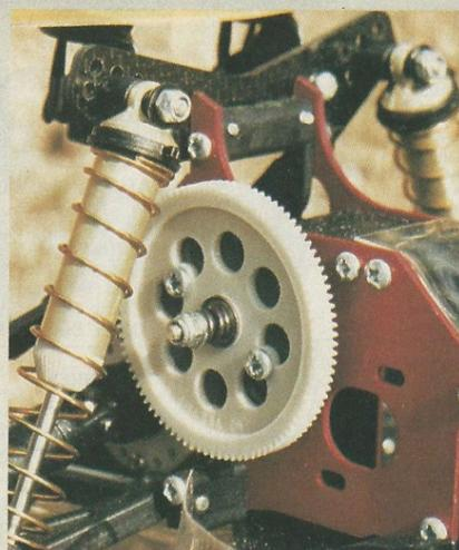
Cougar 2 type 'quick change' slipper clutch can be seen here.
