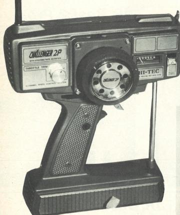
Below: the base of the 'Challenger' case holds the battery pack, eight pen-cells are needed. Ni-Cad batteries can be fitted very easily as the holder connects into an internal charging circuit.
