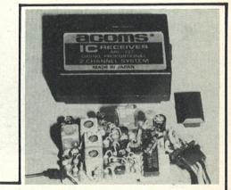
Above: the circuit board of the 'Techniplus receiver displaying a 'forest' of discreet components. Fly leads replace the circuit board block connector which accounts for the greatly reduced size of the unit. Below: the new Acoms servo is a very nicely made unit featuring Acoms own custom built integrated circuit. O-ring sealing is present around the output shaft with rubber sealant
