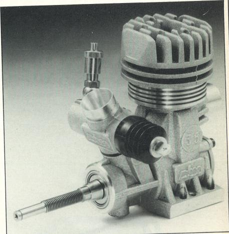
point is also fitted under the main front bearing position, giving the *Picco* the widest mounting base currently available. Use of the one front screw and just two rear ones provides a massively wide and secure triangulated area to hold steady any likely power release (and also makes engine easier to photo!). The Allen grubscrew carburettor mounting bosses held the large 8.6mm slide carburettor rock steady at all rpm points without the continual re-tightening necessary
