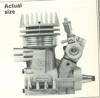
bore to outer face of crankpin. The induction timing now opens and closes some 6° earlier than before.
