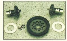
The ball differential is totally conventional in design, and simple to assemble and adjust.
