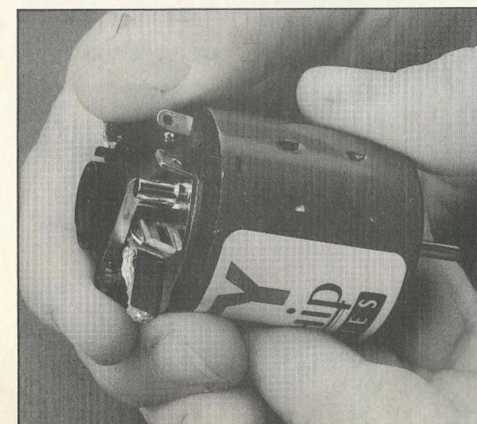
Carefully turn the endbell on the can until it is released.
