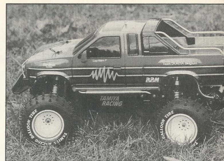
The addition of bolt on rear bars makes the truck look good but they may be a little fragile.
