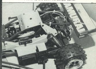
Rear view: the trailing arm rear suspension gives maximum suspension movement although ground clearance on heavy ground under the gearbox may be a problem. All the drive outputs and drive shafts are manufactured in steel whilst power to the rear wheels is through the eternal Mabuchi black endbell 540 motor. Note the difference in tread pattern for the inside of the tyres, possibly to give some semblance of 'toe in' for straight line stability.
