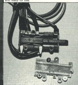
Under view: the space frame chassis is built in two halves and once firmly screwed together with the gearboxes clamped in between forms a very rigid chassis section.
