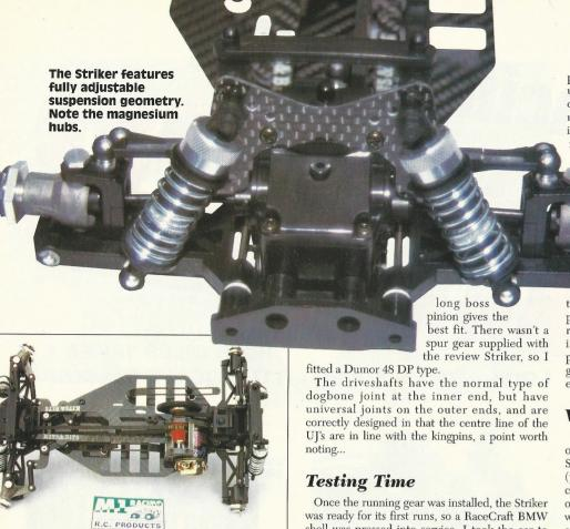
The Striker looks very smart indeed. The use of carbon-fibre throughout for the chassis components and shock towers, plus the black mouldings and alloy parts, give a feeling of real quality. Space is at a premium where the radio installation is concerned.
