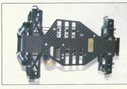
This view of the Striker's underside shows just how small the chassis is in relation to the size of the battery slots. Lovely graphite!
