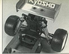
Next are the shocks. Theses are made to the same specification as all the Kyosho shocks but feature a new length front shock, this is a good size and takes care of the suspension movement given by the long front arms. The shocks are really nicely made with particularly nice polished shafts and well moulded pistons.
