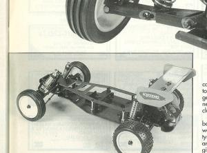
Mid length front shocks specially developed for the Triumph.
