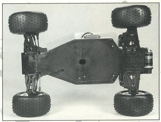
Underside of the car is smooth to allow the car to move easily over rough services. Below; The car has excellent ground clearance and rides the bumps well.
