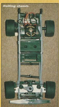
The Kyosho Mini Cooper is a beautifully detailed ½10 scale model of a very classic car from the 1960s. The chassis is of a plastic 'ladder' type design incorporating a standard mechanical speed controller, geared differential, independent front wishbone type suspension and a polycarbonate bodyshell.
