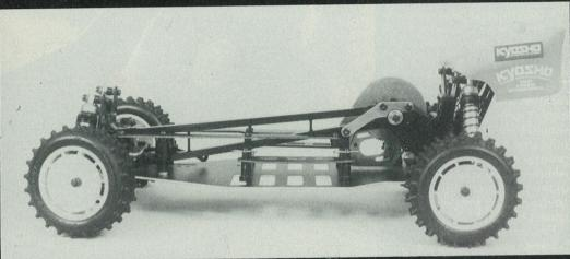
Optima. The new design provides improved ground clearance at the wheel end of the suspension arm. As with the front suspension there is no shortage of adjustments. There are two possible values of rear wheel toe in, made possible by alternative rear suspension pivot blocks. Add to this the top link inner and outer fixing positions and you can finish up with a staggering 240 suspension geometry permutations. Is this over the top?
