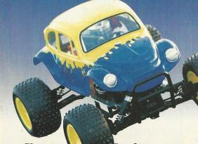
4WD. Shaft Drive. Q.R.C. Gearbox. Twin Geared Diffs Bushed. Dog Bone Driveshafts. Pressed Alloy Chassis & Radio Plate. Kyosho GS11X Engine. Integral Pull-start. Centrifugal Clutch. Engine Driven Cooling Fan. Independent Suspension. Top Link Bottom & Wishbone Front & Rear. Oil Filled Coil Over Shock Absorbers. Dish Wheels. Kyosho Mini
