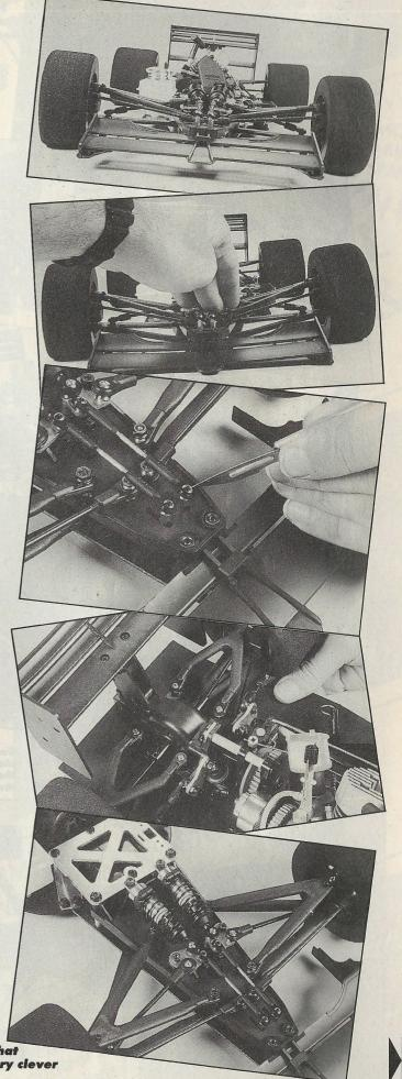
Right: Small amounts of suspension are available but what there is works perfectly. Centre: Front anti-roll bar is very clever using concepts from the world of F1.
