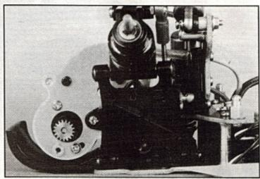
Oinsert a washer here between the wishbone carrier and chassis to give an amount of 'anti-squat'.
