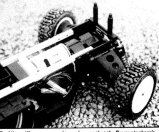
Alloy stiffeners are used to make sure that the Peugeots chassis stays rigid.
