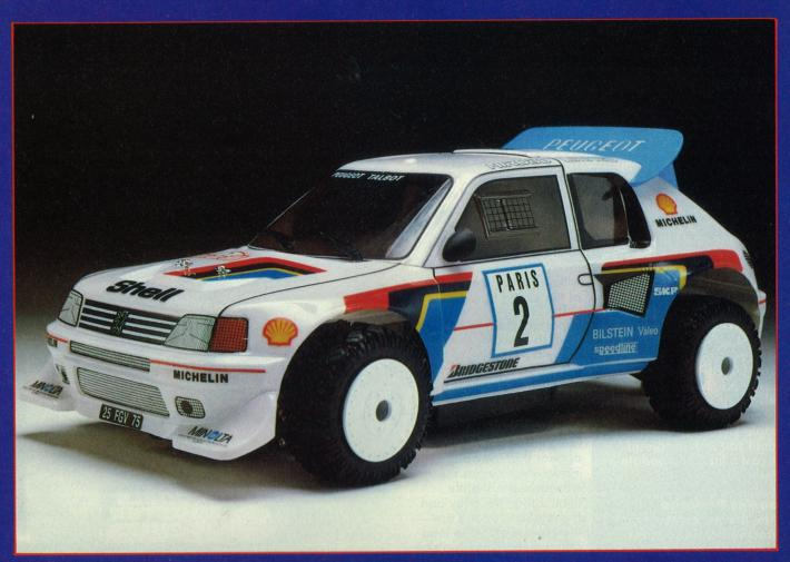
Where the car could be let down, however, is with the chassis which has too much flex for it to be really effective on a race track. For general running, however, it shouldn't be a problem.
