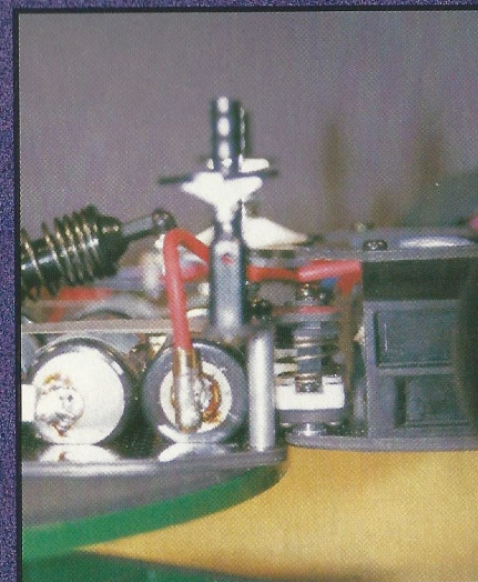
Both the "Roll" control beam and springs can be seen to the left of the alloy pillar.
