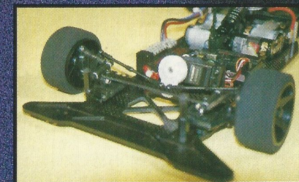
The front suspension of the 10 is nearly identical to the 12.
