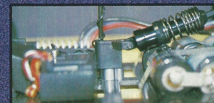
The two alloy spacers under the shock mount can be used to adjust the level of anti-squat.
