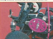
Stock gearing seams fine with a 27 turn motor
