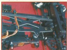
Steering arms are easily adjusted but turnbuckles would have been nice
