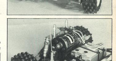
Top right: the overall chassis layout showing Ni-Cad 'stick' pack mounted across the chassis. The GRP plate is cut to fit flush with the body. Tyres are Mardave 'Apache.' Centre right: rear view of the car. The dampers are relocated forward of the axle. The rear of the axle/motor mounts is protected by a piece of clear lexan. Right: close up of the gearbox showing new motor mounting plate and drive gears. This system allows a wider range of quick change gear ratios.
