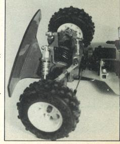
rear end overhung weight and making them less vulnerable to rear impact. Original springs and shockers are used, but with a heavier damper oil and modified piston to cylinder clearances.
