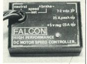
peak of 25A would seem to be fully justified from test results. Obviously with a bypass relay fitted the voltage drop at full throttle was negligible. No plugs or sockets are fitted to the unit, but the instructions are quite specific as to where all the wires go. Of interest it is the only unit which makes special reference to the motor with a 0.1 to 0.3 of capacitor.
