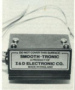
On test the unit gave 0.4V drop at a load of 5 Amps in both forward and reverse directions.
