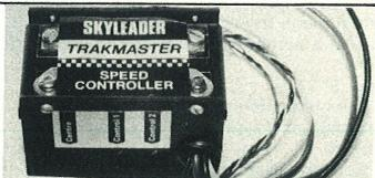
On our fixed 5A load test, we found the unit got warm but not hot. No claims are made as to the maximum running or peak power rating of the unit, but 10A continuous and 20A peak would not seem too unrealistic. We found the volt drop at 5A to be 0.38 Volts. Sizes of the unit 65 × 43 × 41 mm, weight 3.5oz.
