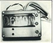
drop of less than one volt at 12A, with a stall current of greater than 25A.
