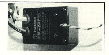
On test naturally with a bypass relay the volt drop was insignificant and it is possible to adjust the point where the relay came in.
