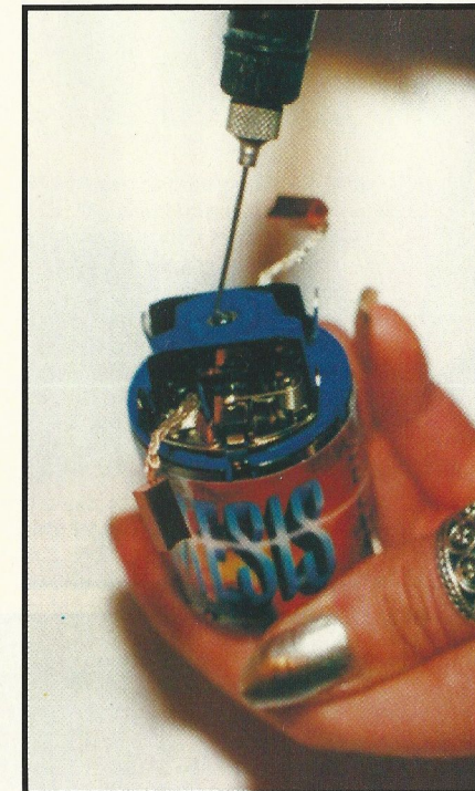
Always re-oil the motor bearings after a re-build, don't add too much.
