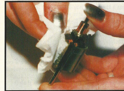
Again clean the com with a soft rag, spraying motor cleaner direct on to the winding can soften the epoxy.
