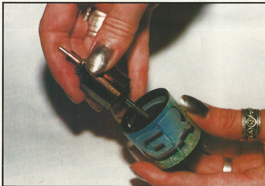
Remove the comm from the can very carefully, note the position of the spacer washers.
