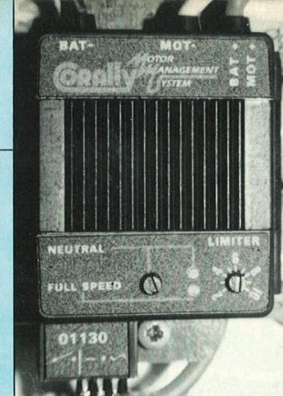
☛ The finned middle section on the MMS II is the all important heatsink to keep the unit as cool as possible. The neutral and torque limit pots can be seen at the bottom of the speed controller.
