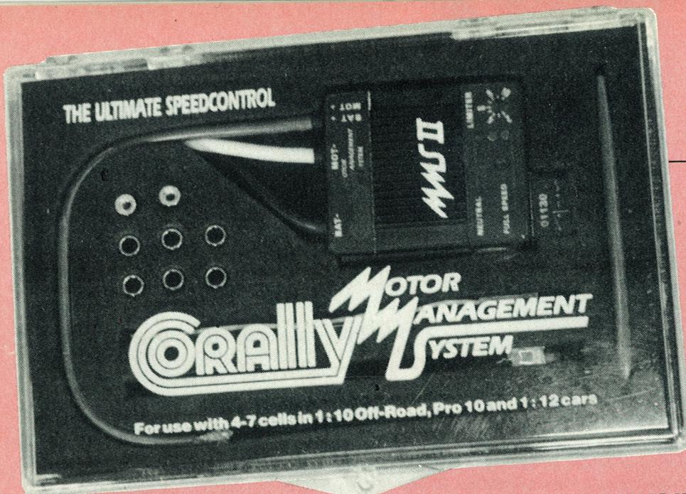
attractive water resistant plastic black case at either side. The neutral and torque adjustment pots are positioned at the bottom of the speed controller, as is the bi-colour LED, which is used for easy setting up of the MMS II.
