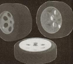
OMki Meteor rear rim with foam on left, Jap 40° foam on Mki rim (centre) and dual compound front tyre with widened Mkl rim (right).
