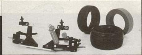
O Another Meteor front end this time with chopped down shock towers, aluminium cross brace and Inboard mounted shocks. This fastidious owner wanted to get his body down lower than everybody else. Shown at right are the new Frewer pneumatic slicks which come complete with foam inners because the soft rubber barely supports the chassis. The weight of the foam is virtually immeasurable. These tyres will fit all the usual rims.
