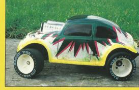
The rounded lexan bodyshell always allows the Digger to finish up on its wheels after a roll. Great paint job by Motion Graphics!
