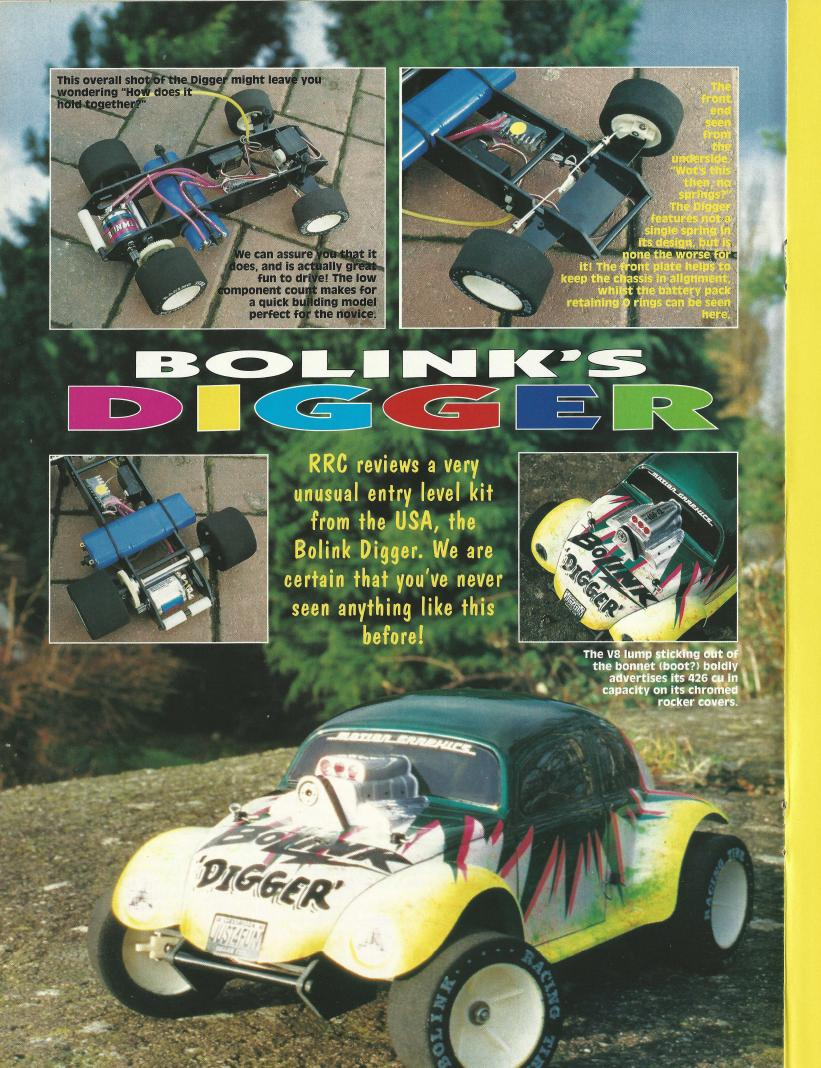
he majority of electric model car kits usually follow a set pattern in their design principles; buggies have a single or twin plate chassis with bulkheads front and rear, on which the suspension arms mount, whilst 1/12 and 1/10 circuit cars usually have all the running gear mounted to a flat chassis plate or 'pan' for simplicity. This little gem from Bolink is of the twin plate design, but in the Digger's case the plates are vertical rather than horizontal!
