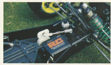
The latest servo saver gives a greater degree of control, having less 'give' than before, whilst the moulded servo mounts prevent the servo itself from moving. Powerful, metal geared servos are advisable!
