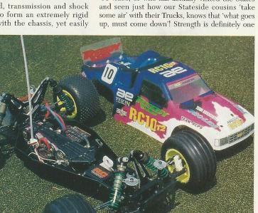
The T2's moulded battery retainer permits the use of either 6 or 7 cells. made up in either stick or saddle pack style. The new design allows much easier use to be made of 'Corally' style connectors.
