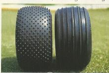
The Pro Line XTR Compound 'Edge' front tyres (right) feature a really novel design to the ribs, whilst the XTR 'Mini Pin' rears are already well known in standard Buggy competition. Foam inserts are supplied for both front and rear.
