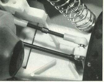
O Turnbuckles are used throughout the car for easy, quick adjustment.
