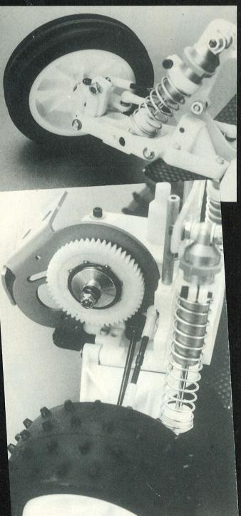
The suspension now features longer top links which mount further inboard on the GRP bulkhead. The reason for this is to lessen the amount of camber change of the rear wheels during suspension movement.
