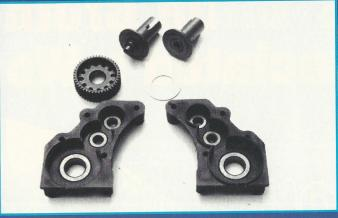
The substitution of baliraces for plain oilite bushings enables the RC10CE to be sold at its bargain price. They're perfectly adequate for outright novices until more speed is required as experience is gained.
