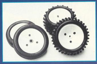
The three-piece wheels allow them to be assembled around the tyres, rather than the tyres stretched over the wheels, which sometimes poses a problem for novices. The tyres supplied are adequate, although are more suited to dirt style tracks than grass.
