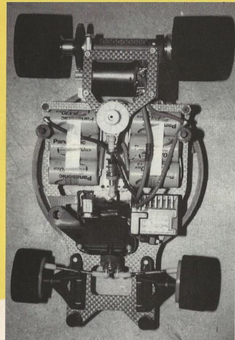
suspension is that it will fit straight onto any 12lw chassis, the only modification required being the repositioning of the (new, longer) front body posts between the suspension at the front. The new chassis now supplied in the kit has two 'ears' or lugs projecting forward at the front on which to mount the posts now that they can no longer
