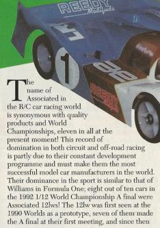
the team have improved the car immeasurably, the latest version being the car pictured, fitted with the new 'wishbone' front end. The rear suspension remains as before, using the conventional T piece and ball set up, this having proved its worth over many years as being rather hard to improve upon.
