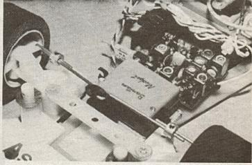
Left: rear pod friction damping system. Above: front end, receiver fits to chassis instead of shaker plate as per usual Associated practice. Below left: alternative hydraulic pod damper. Below right: chassis cut-outs to allow battery suspension.
